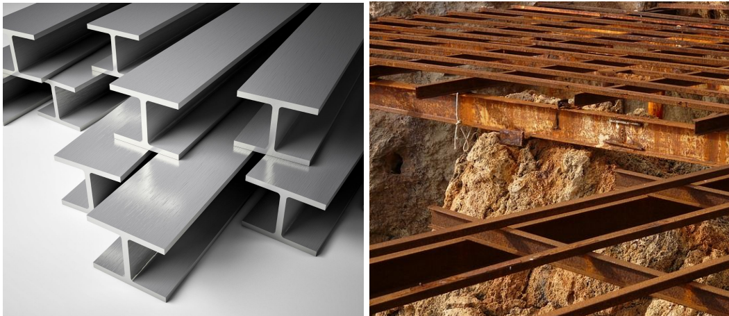
Figure 1. Effect of Corrosion on Steel (“Steel I-Beams”)
