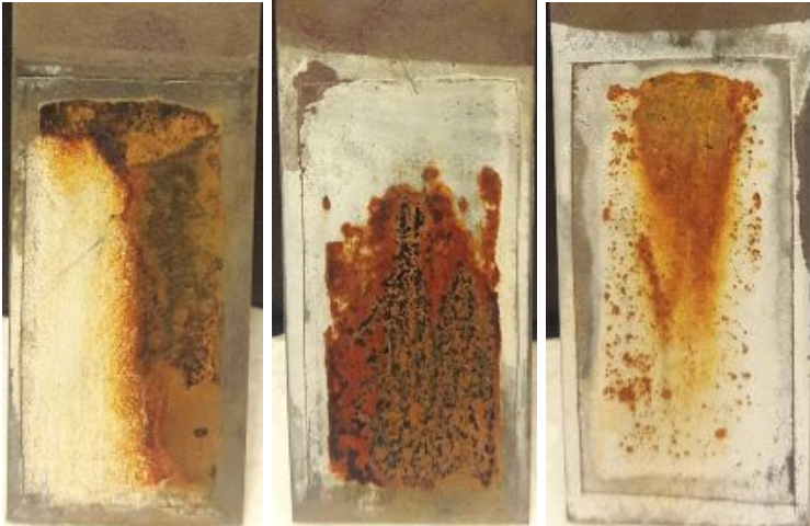
Figure 16. High Potential Difference Trials After Corrosion
